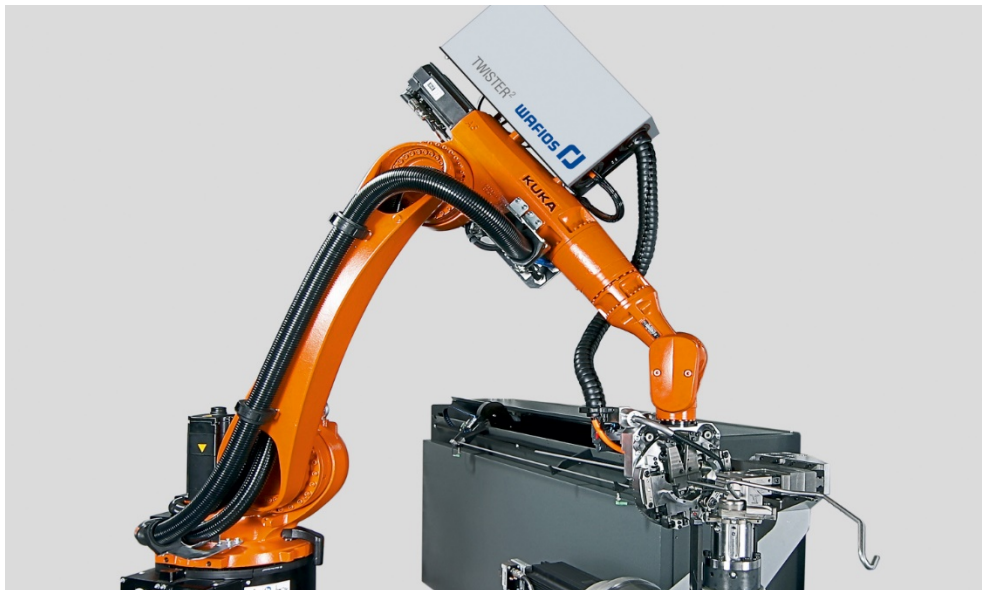
Fig. 2 A highlight of this year's In-House Exhibition is the TWISTER 2 production concept for bending tubes. The WAFIOS programming system WPS 3 Easy Way enables the control of the robot for handling tasks.
