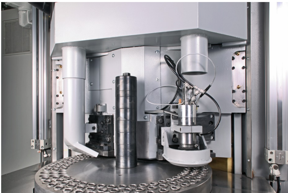
Fig. 2 Active process cooling and "in-process" spring length measurement included as standard in the WAFIOS G 450 series
