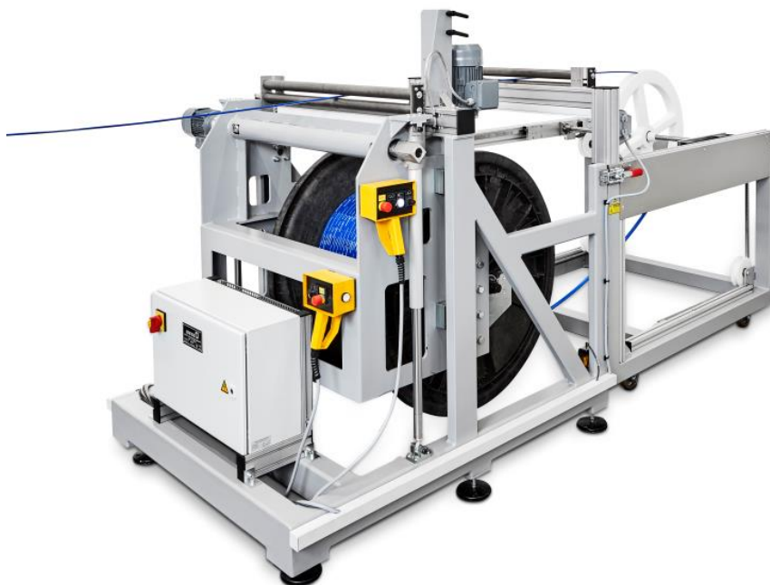
Fig. 3 WAFIOS BMF 60 Pay off for flat material
