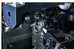
Fig. 3: Feed / guide roller unit, wire cleaning unit and slip control
