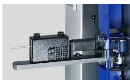
Fig. 3: Feed / guide roller unit, wire cleaning unit and slip control
