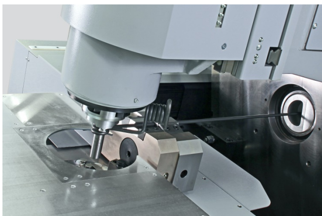
Fig. 2 Coiling unit of a BM 90 single-head wire bending machine.
