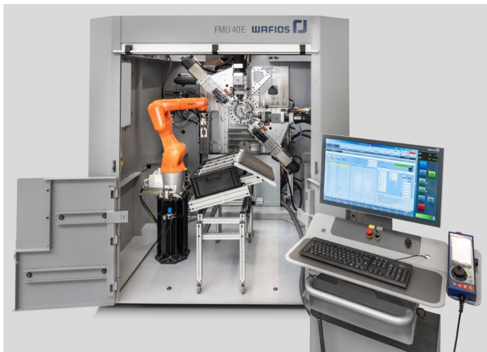
Fig. 3. WAFIOS EasyRobot on FMU 40 E for the production of hairpins
