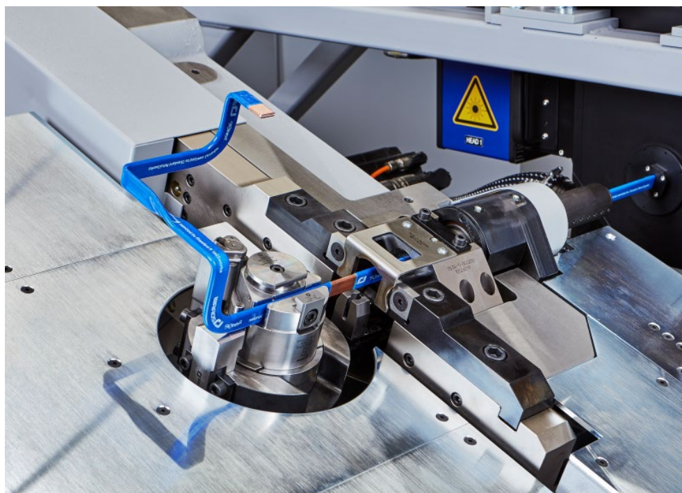
Fig. 4 WAFIOS BMF 60 busbar bending area
