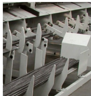
▲ Stop of tilting station and rod-end alignment
