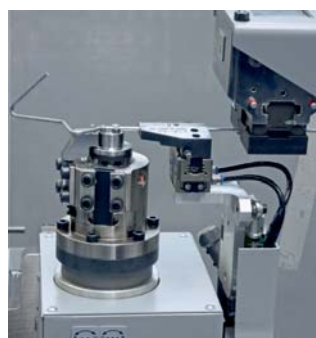
▲ Gripper with swivel arm in connection with bending tool (upper bending head)
