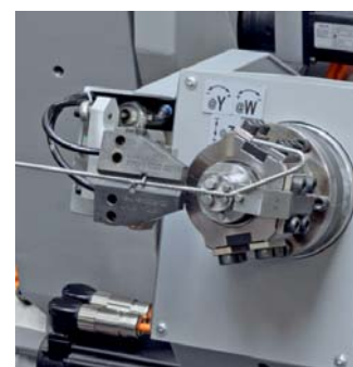
▲ Gripper with swivel arm in connection with bending tool (lower bending head)
