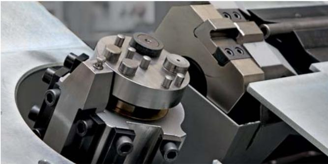
▼ Feed unit including straightening unit
