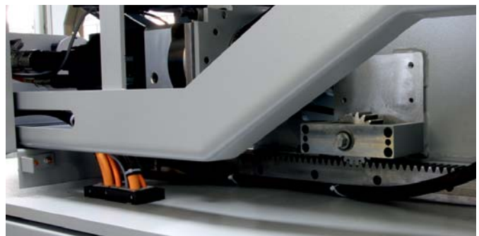
▼ Displaceable feed and straightening unit
