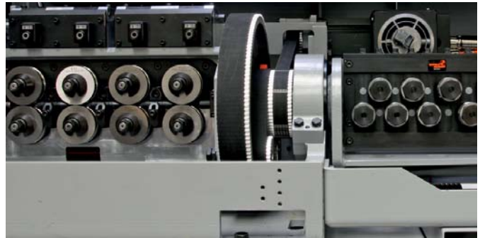
▼ Feed unit including straightening unit
