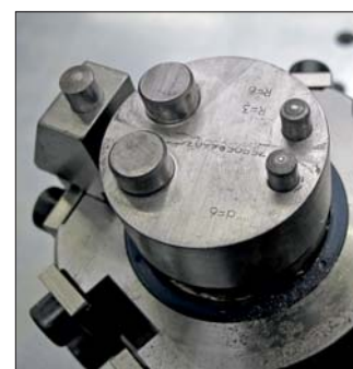
▲ 4-Pin bending tool, type 5
