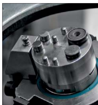
▲ Multi-radii bending tool for bending and free-form bending
