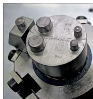
▲ 4-Pin bending tool, type 5
