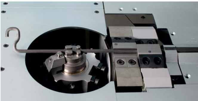
▼ Bending head and cutting unit
