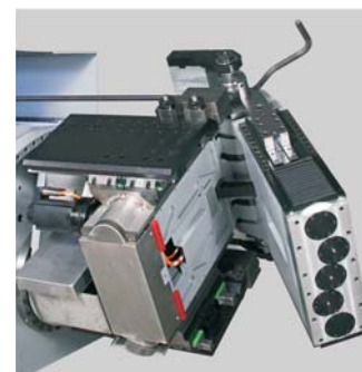
▲ Heavy-duty bending head with closed clamping during bending operation
