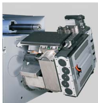
▲ Heavy-duty bending head with open clamping
