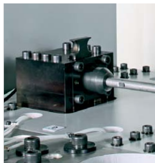
▲ Mandrel bending unit freely programmable over entire tube feed length (patent)
