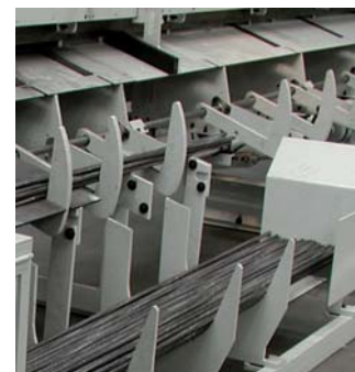
▲ Stop of tilting station and rod-end alignment
