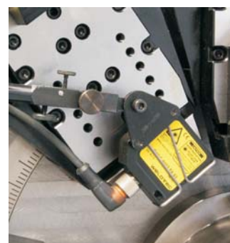
▲ Ejection control with laser
