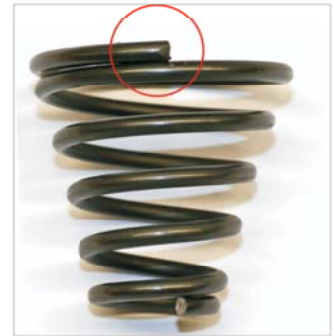
▲ Conical spring produced with PTP coiling finger
