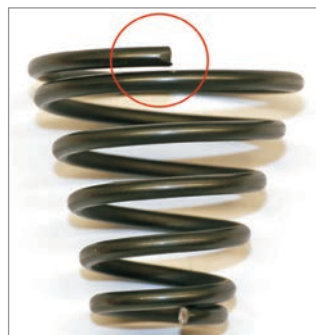
▲ Conical spring produced without motor-adjustable coiling pin holder (PTP coiling finger)
