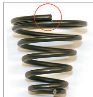
▲ Conical spring produced with motor-adjustable coiling pin holder (PTP coiling finger)
