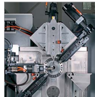
▲ 2-Axis spring and wire forming device FMU 25
