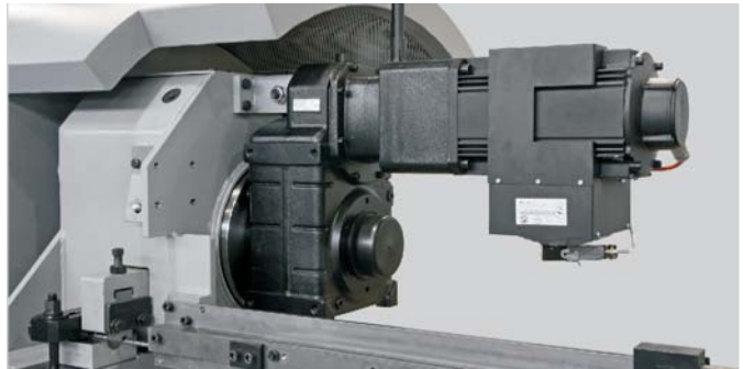
▼ Stationary cutting unit
