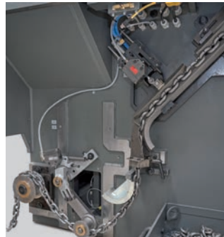
▼ Chain feed with chain feed monitoring and chain brake
