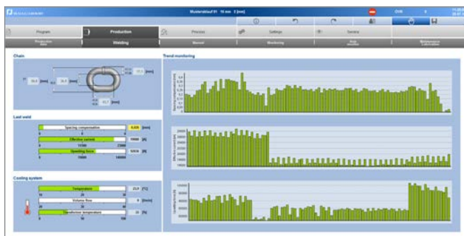
▲ Monitoring of the welding process
